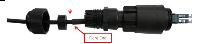
Wrap the rubber split grommet around the jacketing and VERY CAREFULLY push it UNDER the clamping fingers until the grommet is flush with the finger ends. Caution: it will be necessary to gently lift the fingers.
